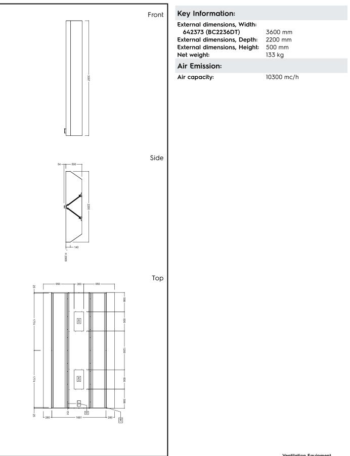
Ventilation Equipment 304 S/S Island Hood+Filters 3600X2200mm
